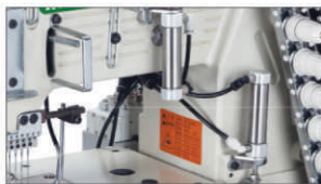
This is the automatic thread blow by air system
