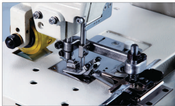
2 needle, flat-bed, making belt loop machine with front fabric cutter and lower puller (the width of belt loop)
