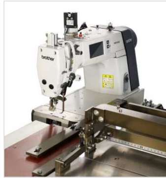
The Brother S-7300A-603P head is used. Ensure the stability of the machine and the beauty of the sewing thread
