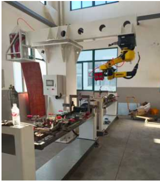
The rack is welded by a robot, and the rack strength is better and the standard is better.
